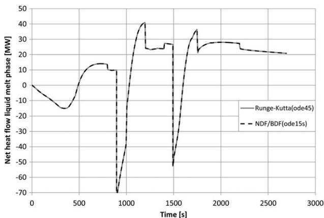
**Figure 7.** Net heat flow to liquid melt for Runge--Kutta(ode45) and NDF/BDF(ode15s).
