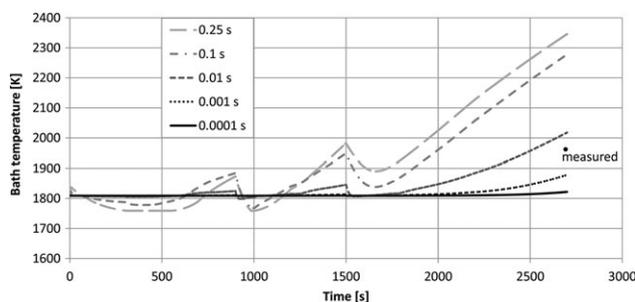
**Figure 2.** Bath temperature calculated with the Euler method.
